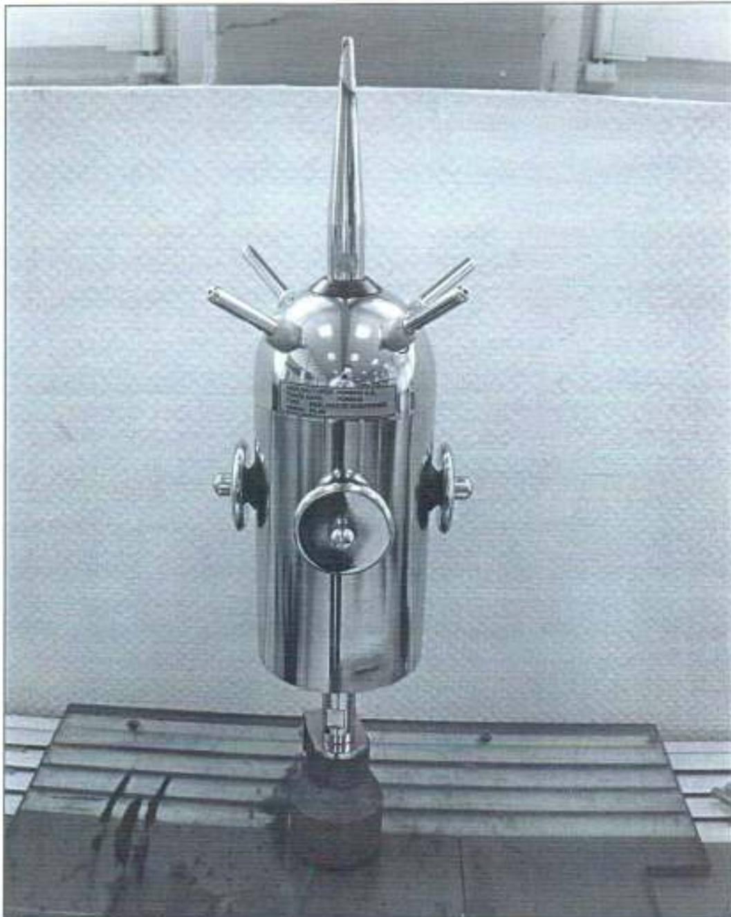
Figure 2: DUT after the impulse current test
